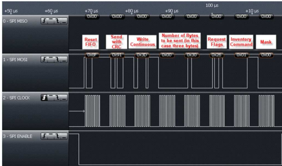
Figure 5-20. Inventory Command Sent From MCU to TRF7962A
