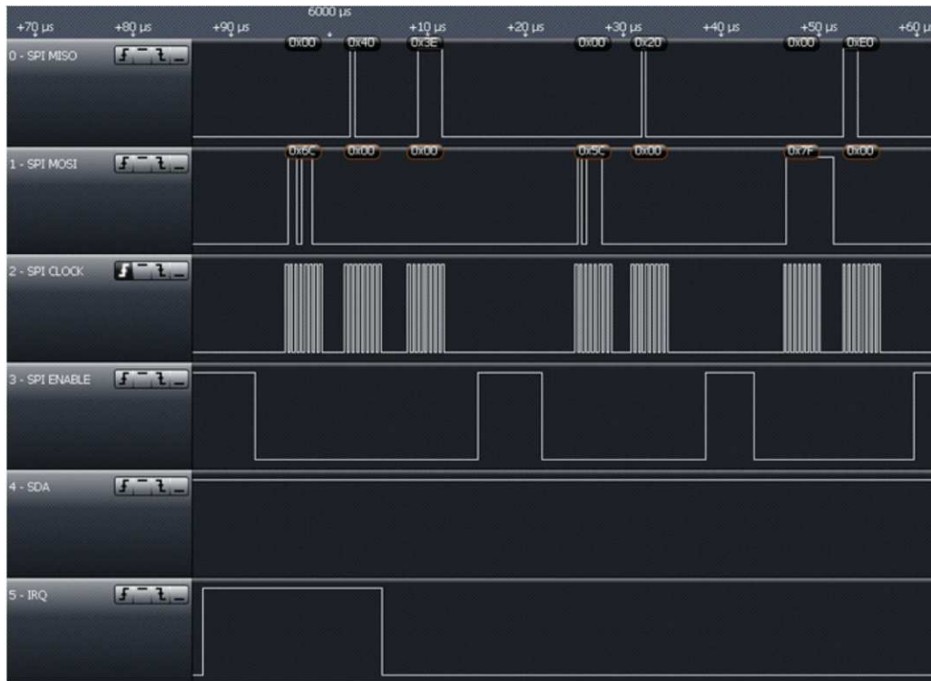
Figure 5-24. IRQ With One Byte in FIFO
